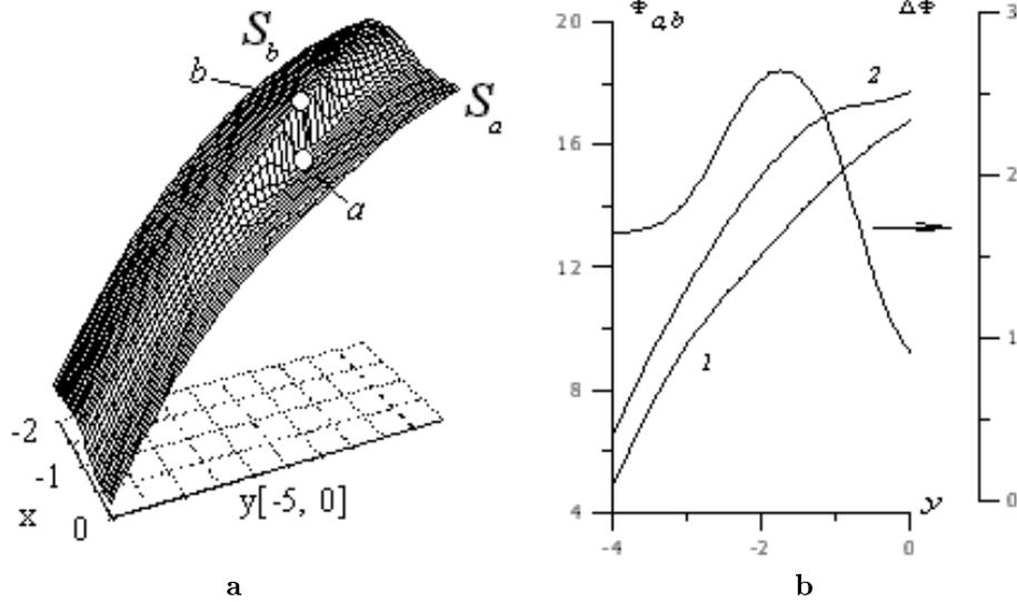
Fig. 5. *a* — structure of the wave front in the area of the tangential velocity disruption of the perturbation velocity; *b* — the wave front  $\Phi_{a,b}(x, y, 1.5)$  phase shift at  $x_a = -0.3$  (1) and  $x_b = -1.2$  (2) (left scale). The phase shift  $\Delta\Phi = \Phi_b - \Phi_a$  (bold curve) between curves 2 and 1 (right scale). Both scales are given in radians
