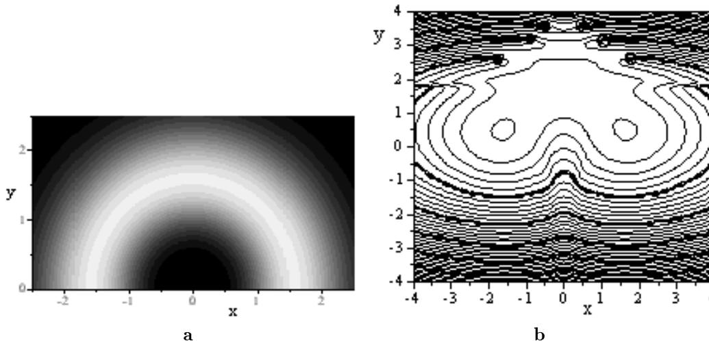
Fig. 4. *a* — beam initial amplitude distribution, *b* — phase map for  $\tau = 0.5$  found with the help of (3). Filled (open) circles correspond to optical vortices with  $m = +1$  ( $m = -1$ )
