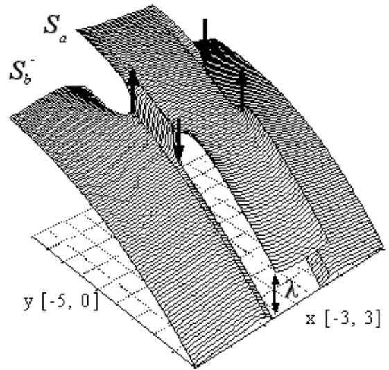
Fig. 6. Structure of wave-front fragments after the switching together phase sheets and the nucleation of the dipoles of vortices. The arrows directed above and down give the location of positive and negative single-charge vortices
