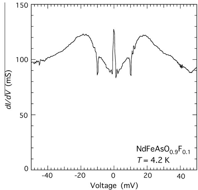
**Fig. 3.** The same as in Fig. 2 but after aging in He vapor atmosphere.
