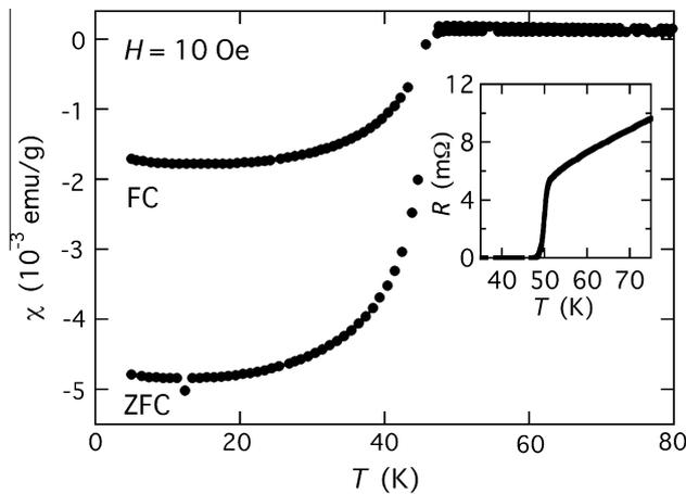
**Fig. 1.** Temperature,  $T$ , dependence of the magnetic susceptibility,  $\chi$ , for NdFeAs(O<sub>0.9</sub>F<sub>0.1</sub>) measured in field-cooled (FC) and zero-field cooled (ZFC) processes. Inset shows the  $T$  dependence of the electrical resistance  $R$ .
