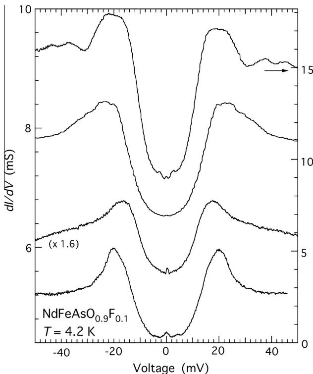
**Fig. 2.** Tunnel conductance,  $dI/dV$ , for NdFeAs(O<sub>0.9</sub>F<sub>0.1</sub>) for several break junctions, BJ, at  $T = 4.2$  K.
