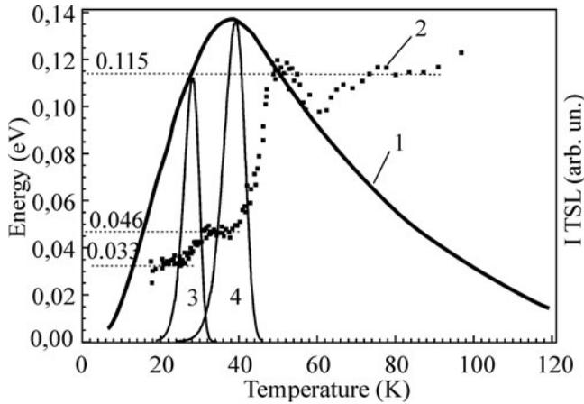
**Figure 7.** TL of PDHS film. 1 - glow curve; 2 - energies of fraction depending on an effective temperature; 3, 4 - glow curves calculated for the energies 0.033, 0.046 eV and  $T_m = 28, 40$  K corresponding to the ends of shelves, respectively [2].
