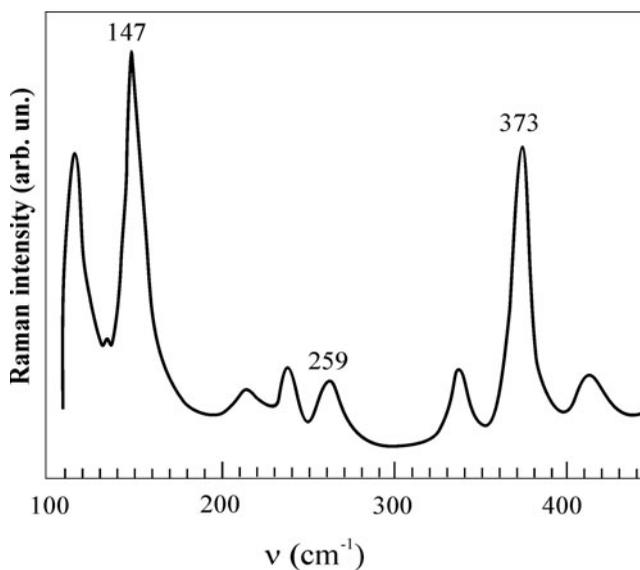
**Figure 5.** Raman spectrum of PDHS powder at room temperature.
