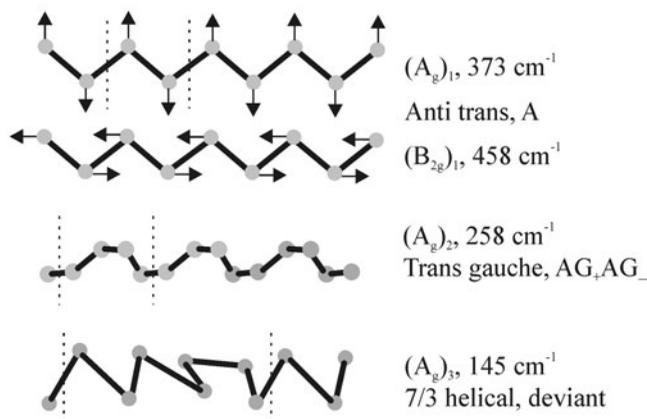
**Figure 8.** Examples of the silicon backbone conformations; dashed lines separates the unit cells.
