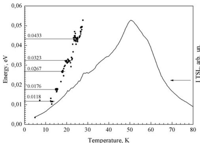
**Figure 1.** TL of PDHS, sample 1. Glow curve (line); fraction energies versus the effective temperature (circles).
