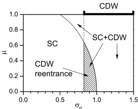
**Fig. 3.** Phase diagram of CDW  $d_{x^2-y^2}$ -superconductor on the  $\mu - \sigma_0$  plane.
