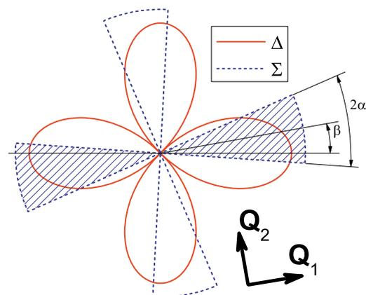
**Fig. 1.** Superconducting ( $\Delta$ , solid curve) and dielectric ( $\Sigma$ , dashed curve) order parameter profiles in two-dimensional momentum space for the bare phases of  $d_{x^2-y^2}$ -superconductor and partially gapped metal with charge-density waves (CDW), respectively, *i.e.* when the competitive pairing channel is switched off.
