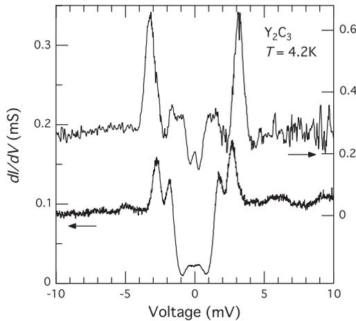
**Fig. 4.**  $G(V)$  for roughly treated  $Y_2C_3$  samples showing multiple gap structures. Curves A and B correspond to different break junctions.
