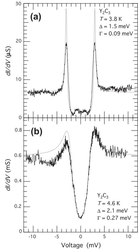
Fig. 2. Tunneling conductance  $G(V)$  for different  $Y_2C_3$  break junctions. The dotted curves were calculated using Eq. (1).
