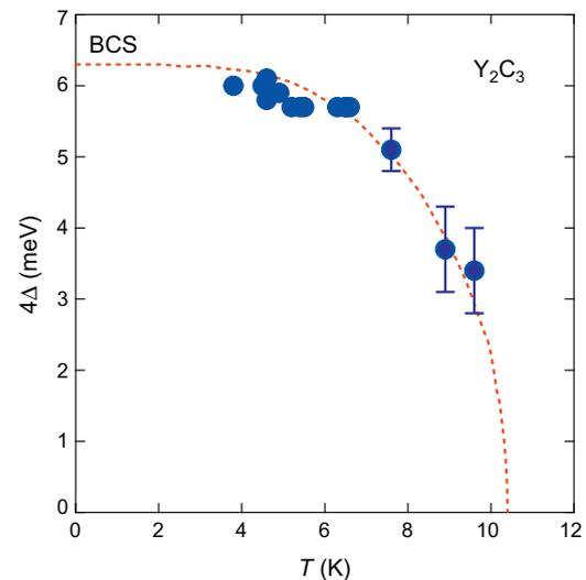
**Fig. 6.**  $T$ -dependence of the peak position  $eV_{p-p} = 4\Delta(T)$  for  $G(V)$  presented in Fig. 5. The broken line represents the BCS prediction.
