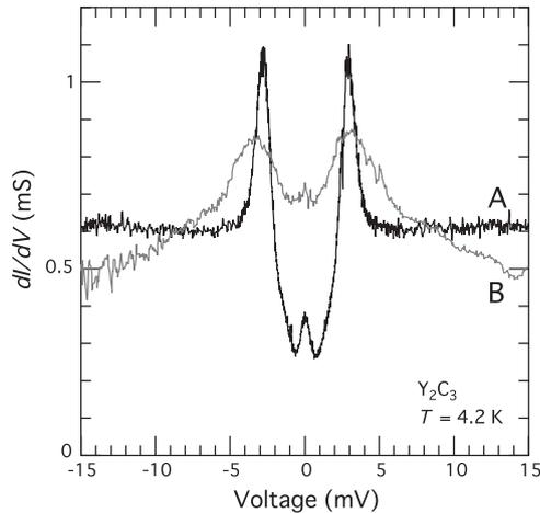
**Fig. 3.**  $G(V)$  for  $Y_2C_3$  measured for a break junction. Curves A and B represent measurements with different external bending forces and, as a consequence, varying interface conditions.
