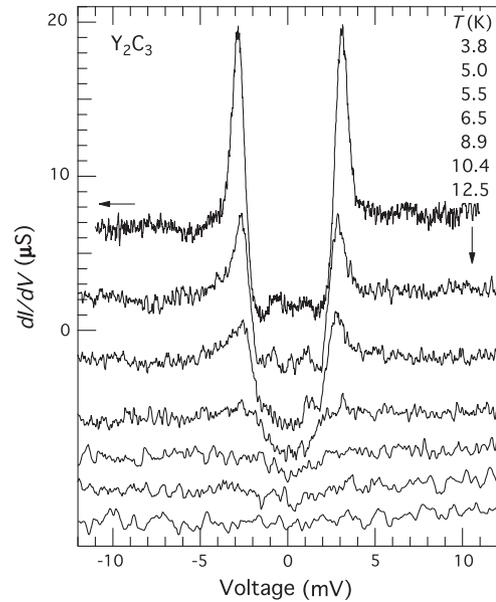
**Fig. 5.**  $T$ -evolution of  $G(V)$  for  $Y_2C_3$ . The junction is the same as that of Fig. 2a.
