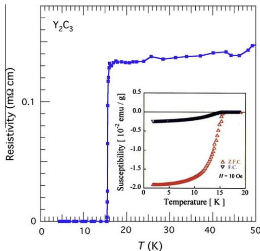
Fig. 1. Temperature,  $T$ , dependence of the resistivity for  $Y_2C_3$ . Inset shows the diamagnetic susceptibility as a function of  $T$ .
