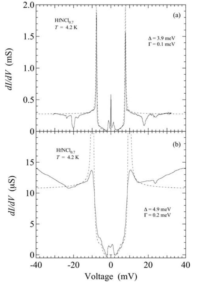
**Fig. 2.**  $G(V)$  for different break junctions made of  $\text{HfNCI}_{0.7}$  at  $T = 4.2$  K. Dashed curves are the calculated BCS conductances for SIS junctions.
